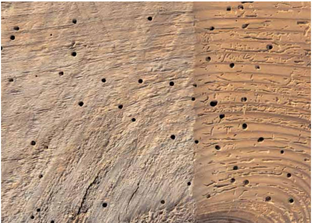
Common furniture beetle – damaged wood (actual size) with, at right, surface partly planed to reveal tunnels
