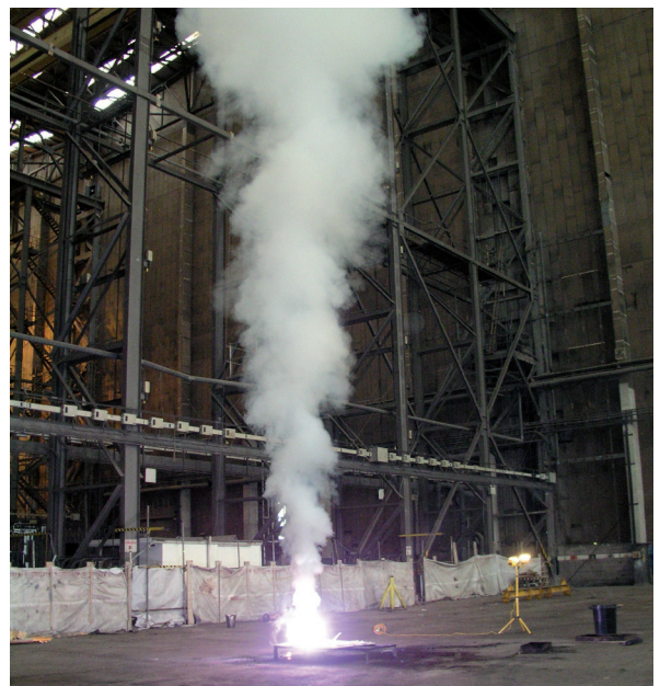
Figure 1: Smoke from the potassium chlorate/lactose performance test fire under way in 43.5 m high hangar
